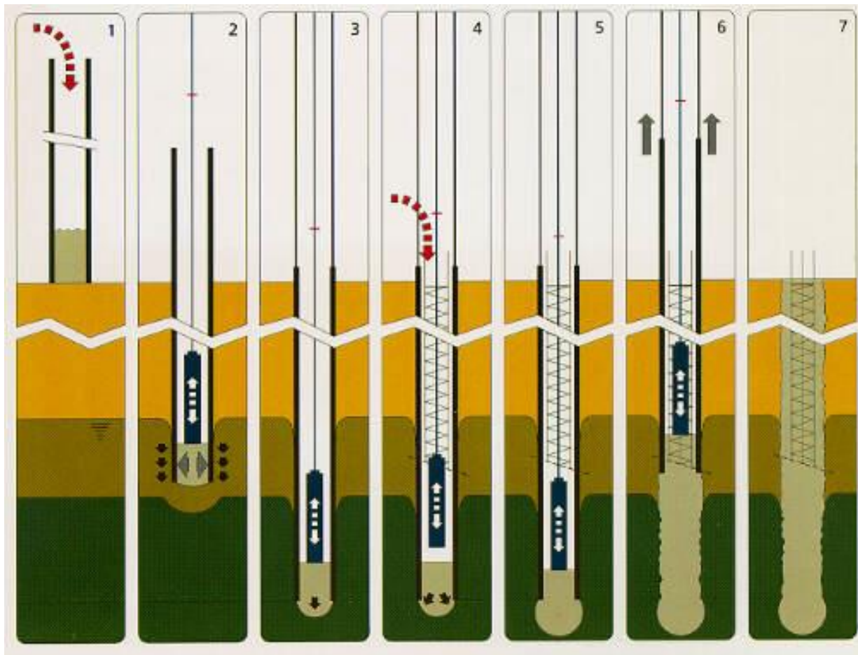
Fig. 57. Construction process of Franki piles
