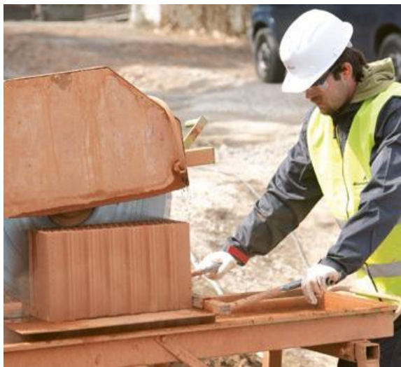
Fig. 23. brick cutting machine
