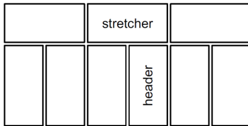
Fig. 10. position of the brick within the wall
